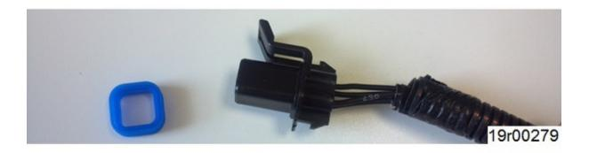
Figure 3, Left: Silicon Seal, Part Number 5348233. Right: Male End of the Engine Wiring Harness Connector.
