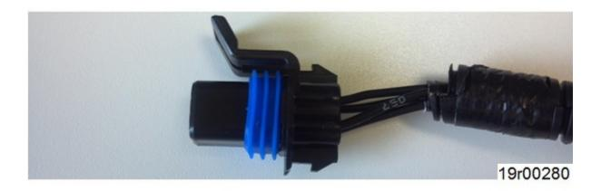
Figure 4, Silicon Seal, Part Number 5348233, Installed On Male End of the Engine Wiring Harness Connector.
