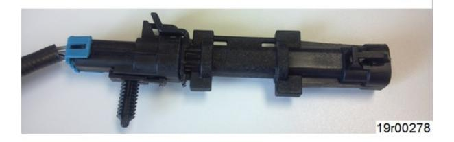
Figure 2, Oxygen Sensor Connector and Oxygen Sensor Wiring Harness Adapter Connected.
