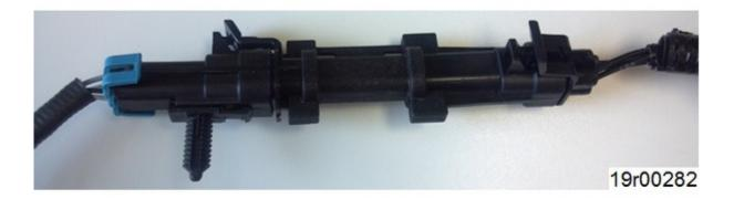
Figure 6, Oxygen Sensor Wiring Harness Adapter Properly Installed.
