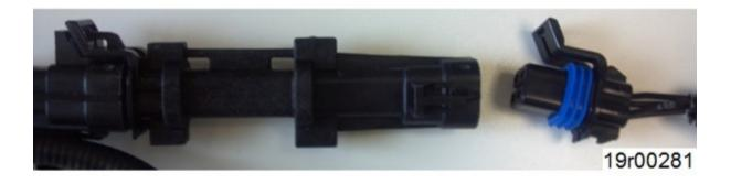
Figure 5, Left: Oxygen Sensor Wiring Harness Adapter. Right: Engine Wiring Harness Connector.
