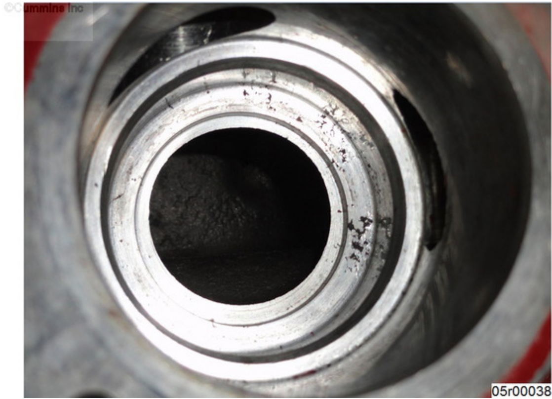
Figure 4, Low Pressure Regulator Bore with Pitting
