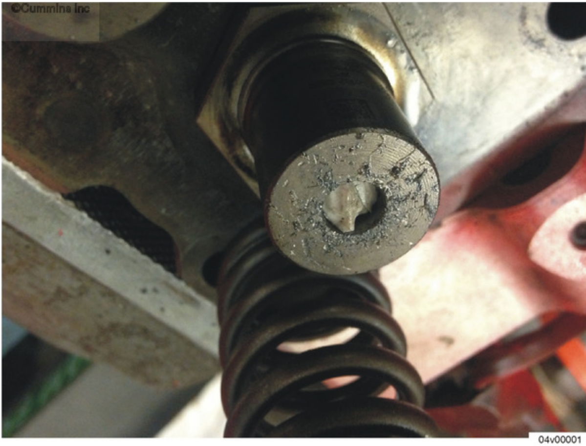
Figure 1: Fractured Fuel Pump Ceramic Pumping Plunger
