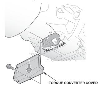
13. Rotate the crankshaft and remove all eight bolts.
