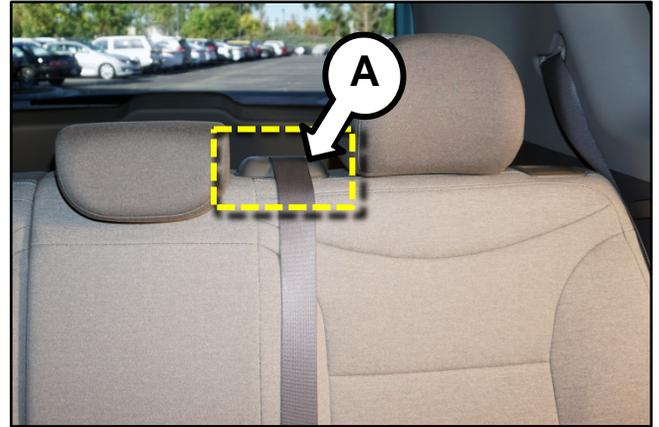
2. Remove the center seat belt guide cover (B) using a trim removal tool, as shown.
