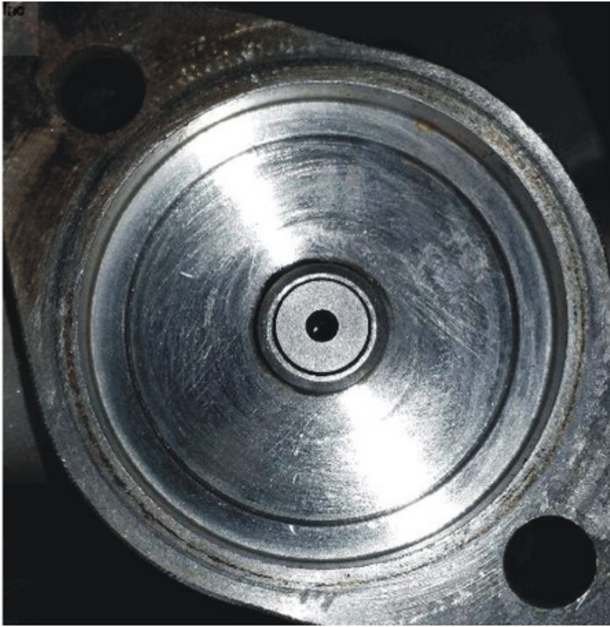
Missing Poppet - EcoFit™ Aftertreatment Fuel Injector
