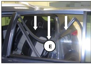
6. Remove the door molding from both sides and replace them with new ones (F).
