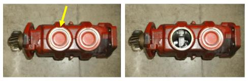
2) Rotate crankshaft so that the date code on the crankshaft if visible.
