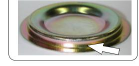
3. Press the plug in the crankcase until the flange of the plug seats to the crankcase shoulder.
