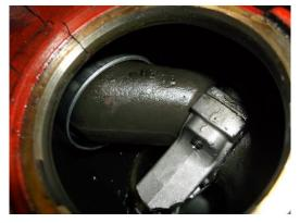
3) With a flashlight, review 4 digit casting on crankshaft. IF those digits are "22/12" or earlier, then compressor must be replaced. Otherwise, continue to next step. (Ex: The picture below has a crankshaft date code of "18/10" therefore, it would need replaced.)
