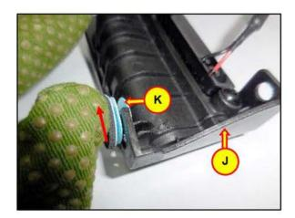
11. Reuse the clip (K) for the new switch assembly (J).
