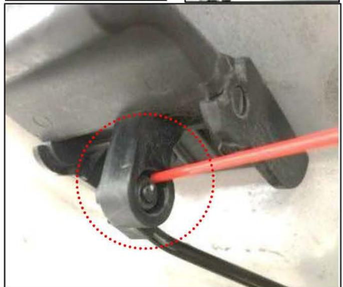
3. Verify proper operating of secondary hood latch. Wipe off any excess lubricant.
