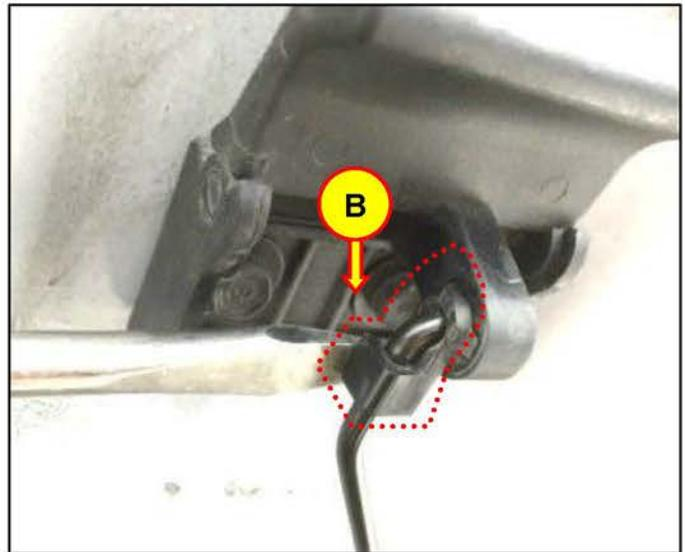
3. Install the new secondary hood latch in the reverse order of removal. Verify proper operation of the secondary hood latch while opening and closing the hood. Ensure the secondary hood latch keeps the hood from opening unless the secondary hood latch release is activated.
