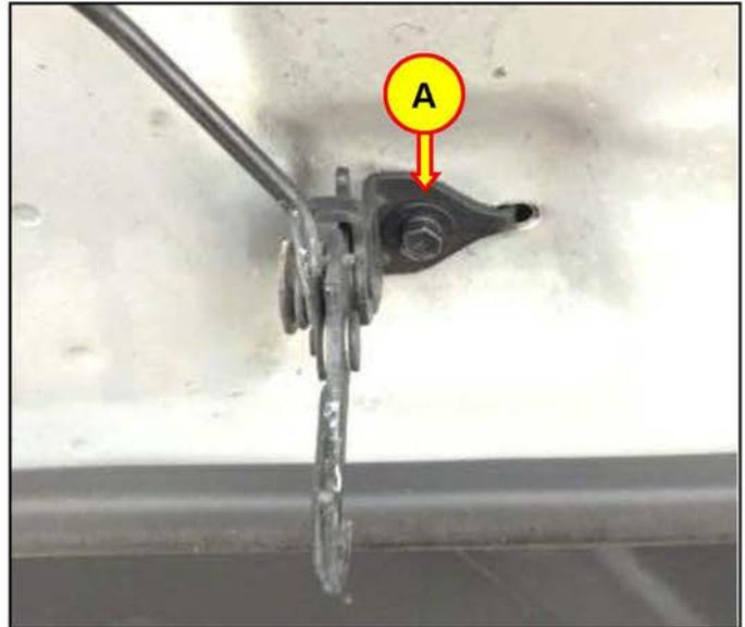
2. Unlatch clip (B) from the rod connected to the secondary hood latch release lever. Then remove the rod and secondary hood latch assembly from the release lever.
