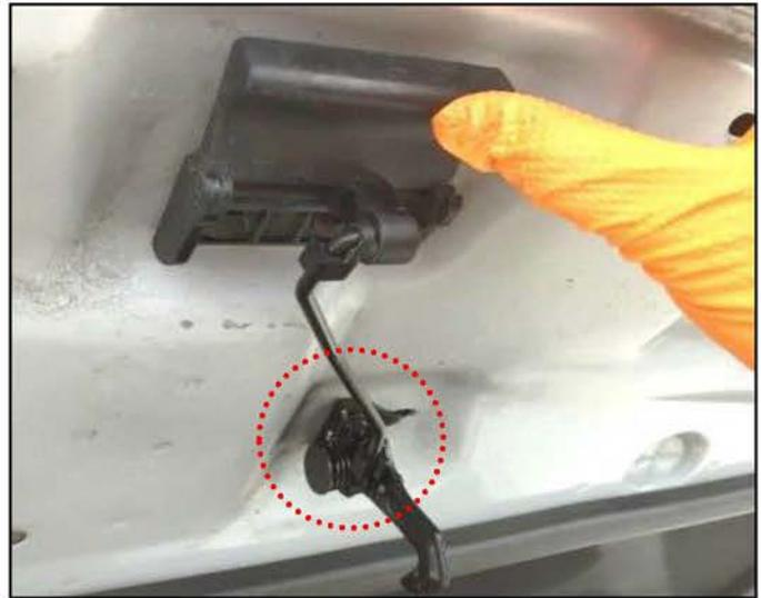
2. Apply a sufficient amount of WD-40 Specialist lubricant onto rod, riveting area, and clip.
