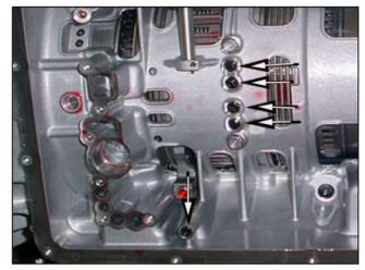
Carefully align the manual valve to the shift lever and reinstall the valve body.
