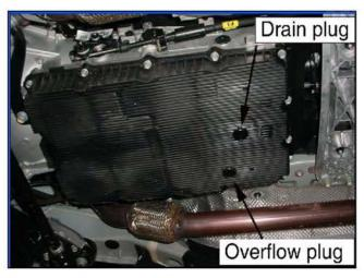
ATF TEMPERATURE = 122~140°F (50~60°C) SHIFT LEVER IN "P" AND ENGINE RUNNING
