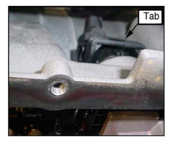
Use an 8mm or 5/16" hex socket and remove the drain plug and drain the ATF. Reinstall the drain plug.
