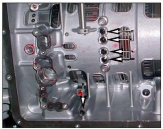
Carefully align the manual valve to the shift lever and reinstall the valve body.
