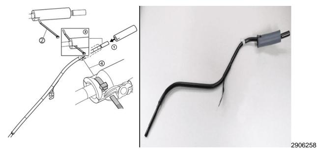
**Note:** The tie strap threads between the fill tube and half the foam damper using the slot in the sleeve. This is secured to the top half of the tube, leaving the lower half of the damper free.
