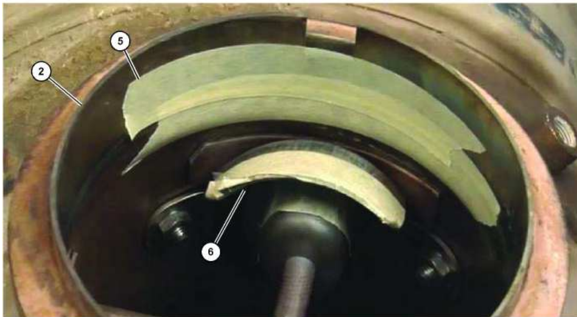
Illustration 9 (2) SCR catalyst outlet pipe (5) Masking tape (6) Outlet NOx sensor internal water shield
