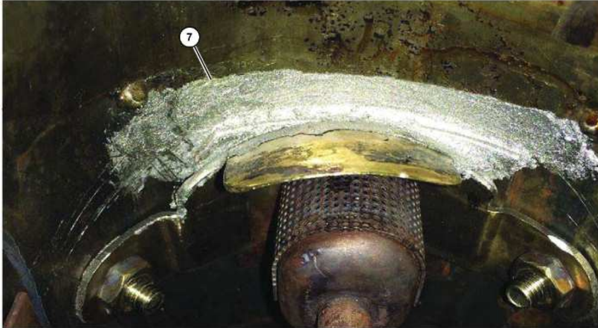
Illustration 12 (7) High temperature sealant
