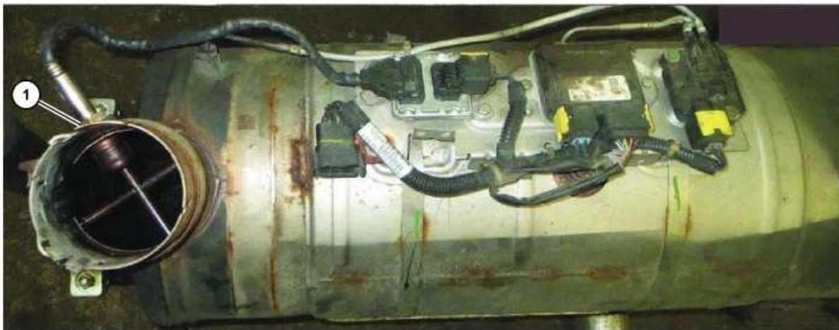
Illustration 1 (1) Outlet NOx sensor
