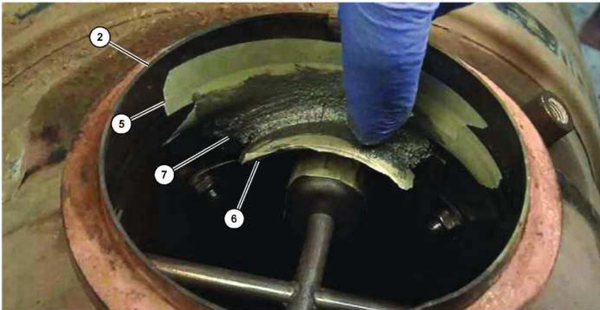
Illustration 11 (2) SCR catalyst outlet pipe (5) Masking tape
