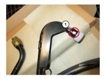
Illustration 1 g06042616 Verify the white marking on the end of heater pipe in call out 1
