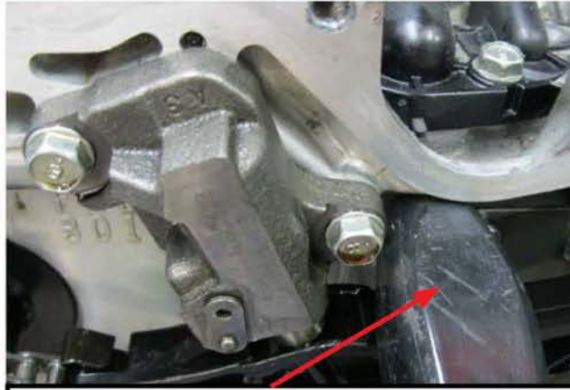
Plastic screw driver handle inserted between front lip of the block and the B2 upper chain guide VERY CAREFULLY pushing downward on the upper guide.
