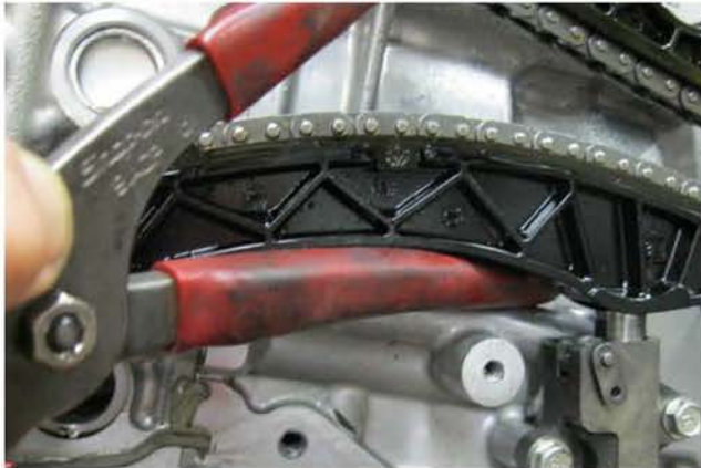
Rubber-coated plier handle inserted between a ledge area on the front of the block and the B1 lower chain guide VERY CAREFULLY lifting upward on the lower guide.
