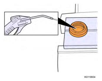
10 Ensure the drain hole in the bottom of the exhaust rocker compression brake piston housing is clean and clear of any debris.
