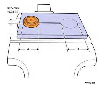
5 Secure the exhaust rocker compression brake piston and the retainer tool in the vise.
