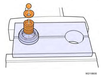
11 Install the internal components in the exhaust rocker compression brake piston housing.
