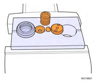
8 Using brake cleaner, clean the internal components and the threads on the cap. Store the internal components and cap in a secure location for installation.
