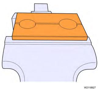
3 Measure the diameter of the exhaust rocker compression brake piston to determine the appropriate tool opening to be used in this repair procedure.
