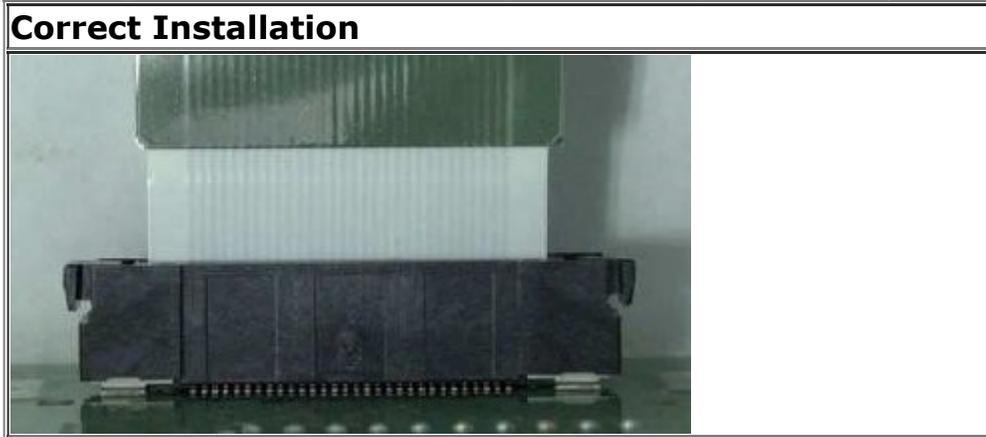
**Caution:** Do not force out/insert the wiring harness end without pushing the tabs, or the wiring harness end hook(s) may be damaged. If the hooks are damaged, the AD-Disp may not operate because of a loose and/or incorrect fit of the wiring harness end.
