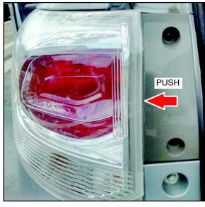
b. Push the rear combination lamp to the outside by hand until the clearance between the tailgate garnish and rear combination lamp is more than 5 mm.
