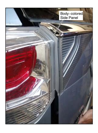
Open the tailgate and hold slightly away from car until the body—colored side panel of the tailgate garnish is visible.
