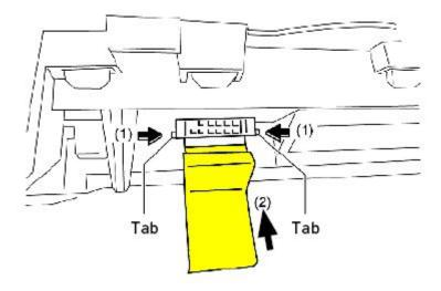
**NOTE:** Verify that the wiring harness end is inserted straight and securely locked in the position as shown below.
