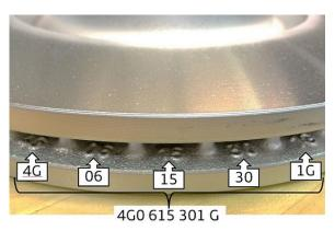
Figure 3. Front brake disc part number location.
