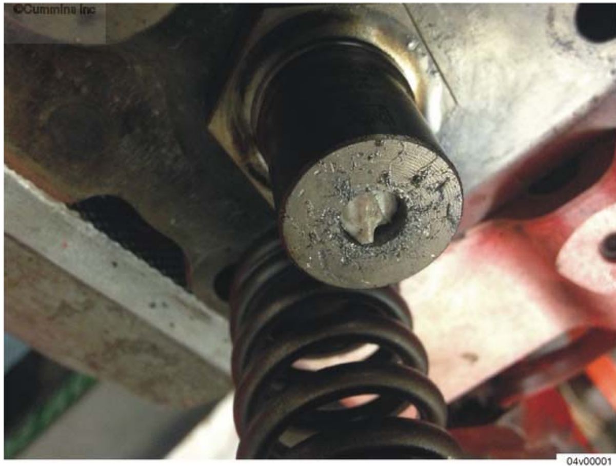
Figure 1, Fractured Fuel Pump Ceramic Pumping Plunger.
