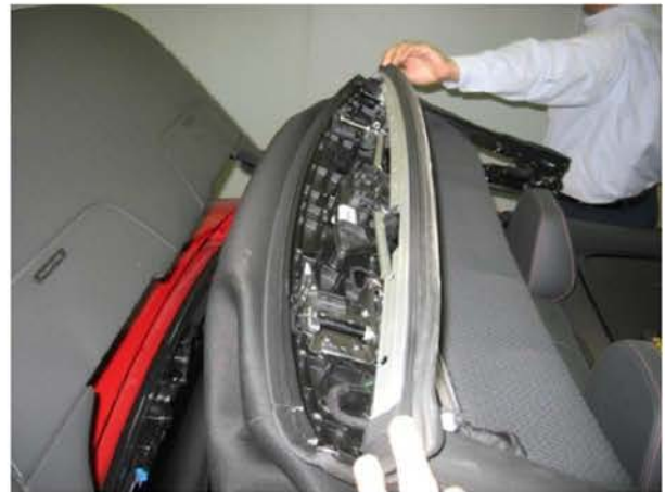
Figure 5. Retaining strip and seal pulled back.
