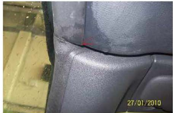
Figure 2. Evidence of a leak.
