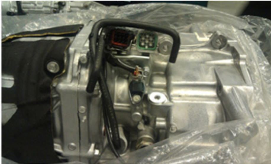
Bracket attached, CVT ready for installation.
