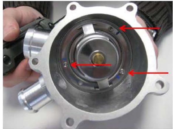
Figure 1. Remove the three Allen screws (red arrows) to remove the thermostat.
