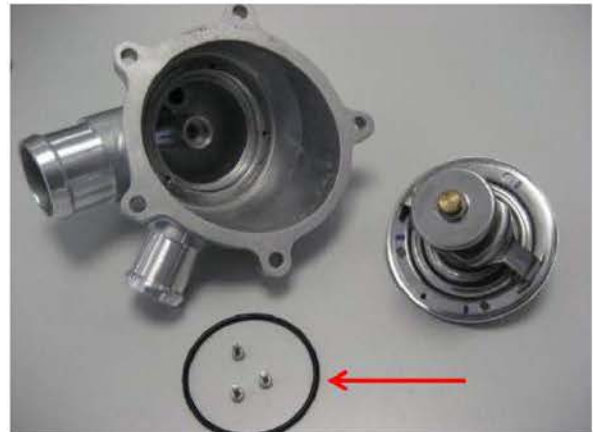
Figure 2. Thermostat housing seal (red arrow).
