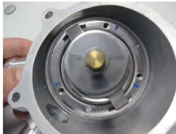
Figure 4. New thermostat installed.
