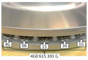
Figure 3. Front brake disc part number location.
