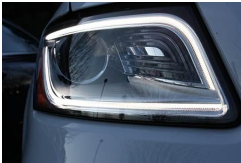
Figure 1. Upper and Lower light pipes illuminated.
