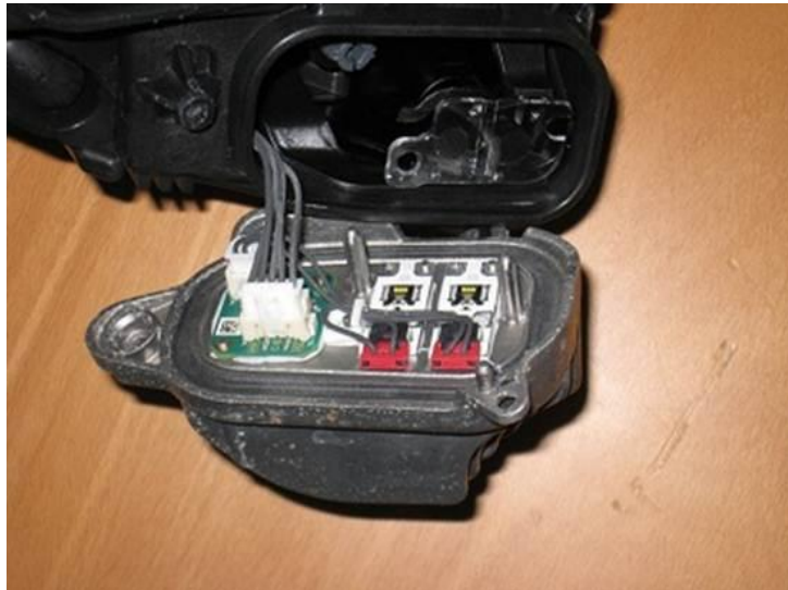
Figure 7: Dual surface mount LED unit exposed.
