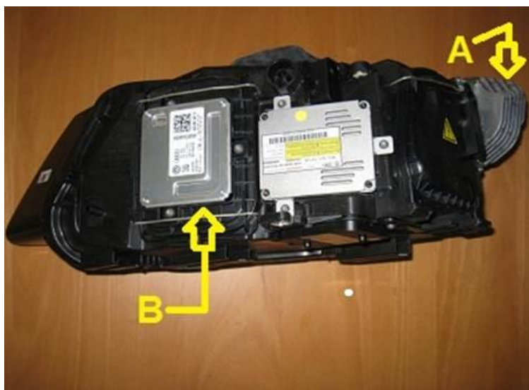
Figure 2. Backside of headlight with LED heat sink (A) and LED control module (B).
