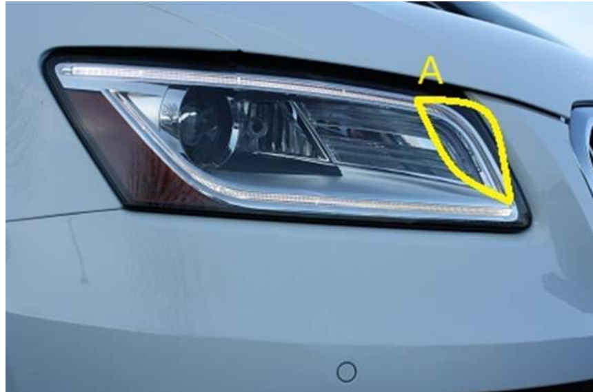
Figure 5. Upper light pipe perceived defect (A).
