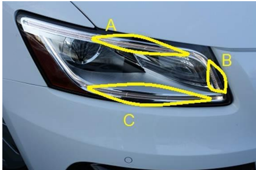
Figure 6. Upper light pipe perceived defect (A, B). Lower light pipe perceived defect (C).
