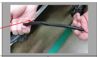
Strip ¾" of casing off both wires that have been cut. Twist the orange/white wires together and the two black wires together and solder.
