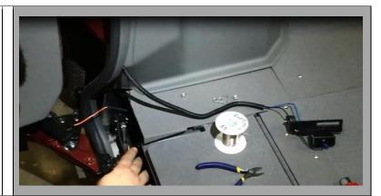
3. Using a reciprocating saw or another suitable tool cut out the end of the slotted hole in the rail as shown. Make sure surface doesn't have any sharp edges left after the rail is cut.
