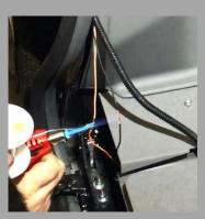
10. Move heat shrink into position and heat evenly until no gaps are between wire and heat shrink. Once cool, slide loom casing back over wires and re-install into the panel. Be sure the weather-strip is replaced and set.
