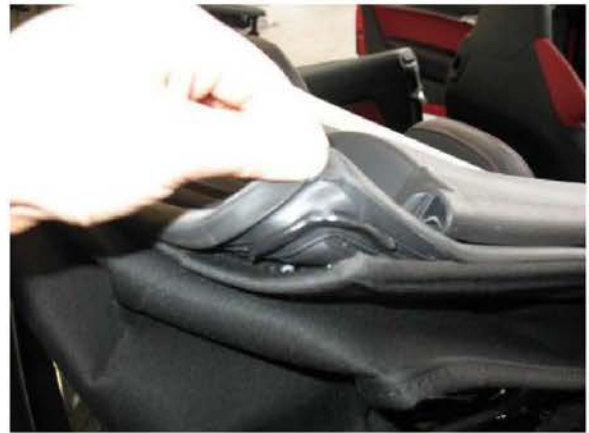
Figure 7. Pushing excess butyl cord into the end chambers.
