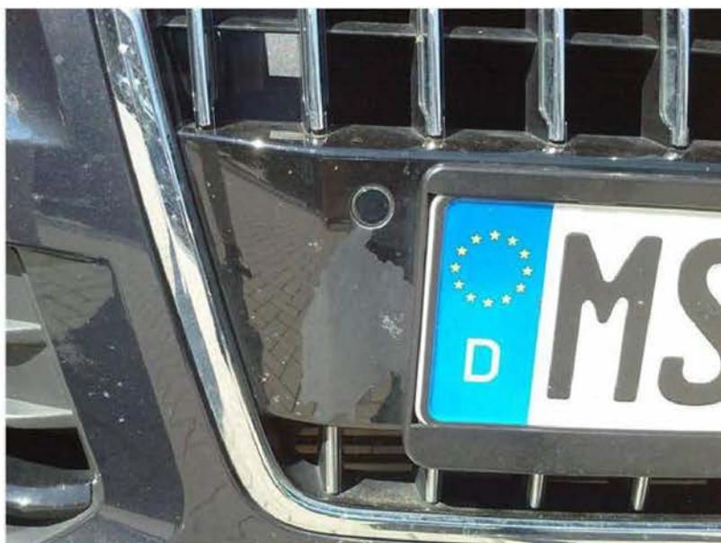
Figure 1. Example of flaked-off paint.
