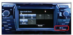
B. Push the Map Micro SD Card to eject it from the slot.
