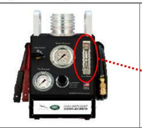
The high-pressure diagnostic leak detector has a variety of applications in detecting even very small leaks in different applications
