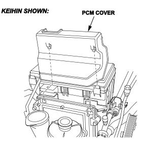
31. Remove the PCM connectors and harness clip. Remove the battery cables from the underhood fuse box.
