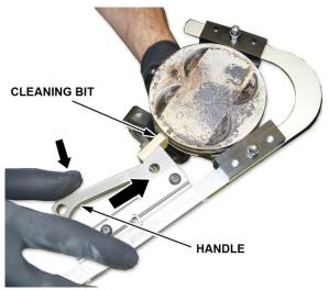
5. Once the cleaning bit is in the appropriate ring grooves of the piston, make sure the tool handle clicks in to place. NOTE: There is only one notch on the tool for the handle to engage.
