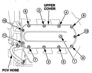
29. Remove the intake manifold bolts and nuts in three steps, then remove the intake manifold.
