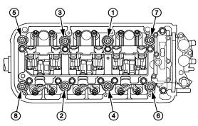
41. Measure the head bolts to determine if they need replacement. If either diameter is less than **11.3 mm (0.445 in)**, replace the cylinder head bolt.
