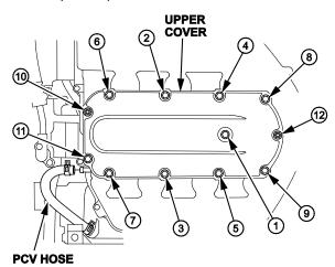
29. Remove the intake manifold bolts and nuts in three steps, then remove the intake manifold.
