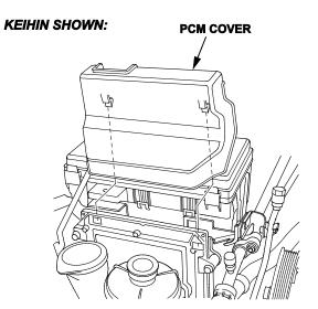
31. Remove the PCM connectors and harness clip. Remove the battery cables from the underhood fuse box.
