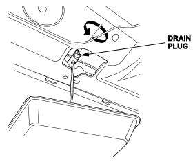
11. Install a 5/16th inner diameter rubber hose on the drain bolt located at the rear of the engine block, loosen the drain bolt, and drain all remaining coolant. Then disconnect the oil pressure switch connector.
