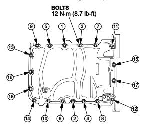
46. Using a flat blade screwdriver, separate the oil pan from the engine block in the areas shown.
