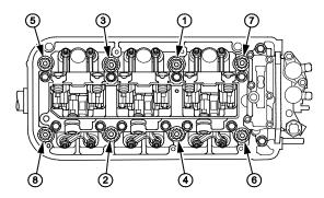
41. Measure the head bolts to determine if they need replacement. If either diameter is less than 11.3 mm (0.445 in), replace the cylinder head bolt.
