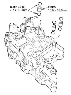
3. Transfer the 14.3 mm x 37 mm pipe into the new valve body with new O-rings and with the filter end facing the valve body assembly.
