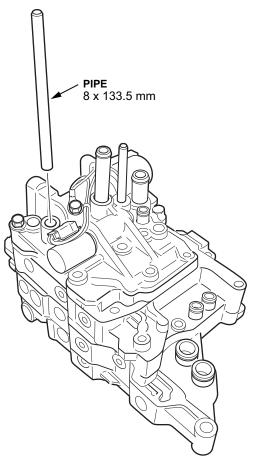
7. Transfer the 10.9 mm x 25.5 mm pipe into the new valve body with new O-rings.
