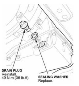
4. Reinstall the drain plug with a new sealing washer.
