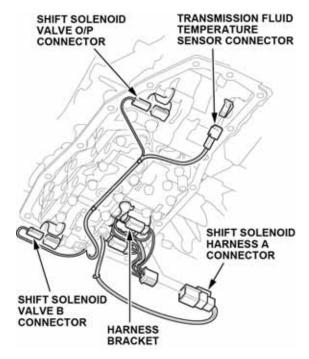
9. Remove the guide plate, then remove the lower valve body assembly.
