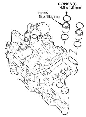
2. Transfer the 10.9 mm x 18.6 mm pipes with new O-rings into the new valve body.
