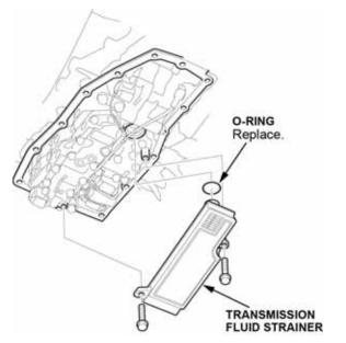
7. Inspect and clean the inlet opening of the transmission fluid strainer as needed. Replace it if it is clogged or damaged.
