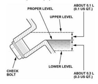
17. .Reinstall the check bolt with a new sealing washer.
