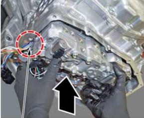
Be careful not to pinch these wires as the valve body is pushed upward.
