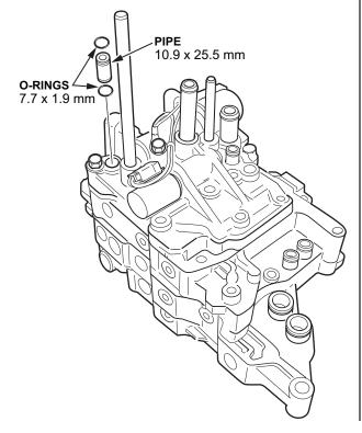
8. Install the new lower valve body assembly and the bolts. Tighten them in a crisscross pattern in at least two steps
