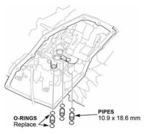
16. Remove the two 18 mm x 18.5 mm pipes and the O-rings.
