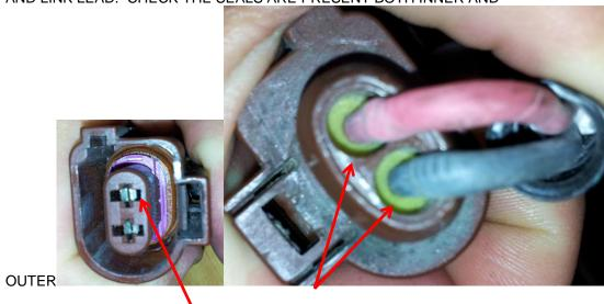
LINK LEAD SEALS – INNER AND OUTER. CHECK FOR PRESENCE AND DAMAGE.
