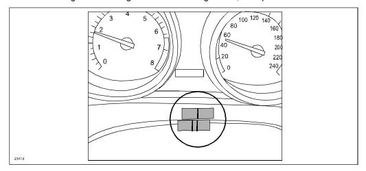
4. Measure the distance between the two lines. The offset can be approximately calculated using 1mm = 1° of offset.
