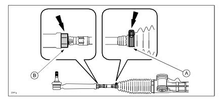
3. Rotate the tie-rod to adjust the steering wheel center. Refer to the following charts for rotating direction.
